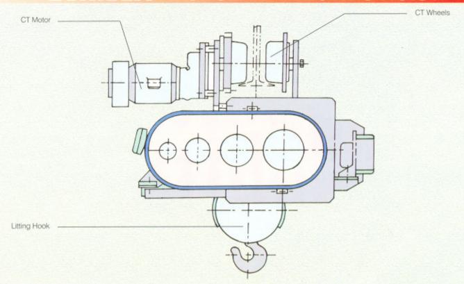
**Trolley:** The hoist trolley is underslung type drive for straight travel on beam. Flexible trolly suitable for curved path can also be supplied. All trolleys are adaptable to large range of flanges of rolled beams or fabricated beams or box sections.
