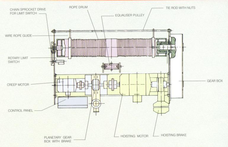
DESIGN: ELMECH Hoists are designed for heavy duty and high duty functional value. These are compact and are specially developed for Steel Plant Industries. All ELMECH HOISTS are designed conforming to IS:3938, FEM Std and DIN Specification.
